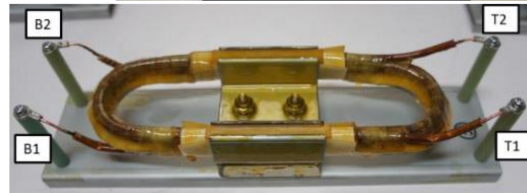
Motorette sample with varnish treatment
